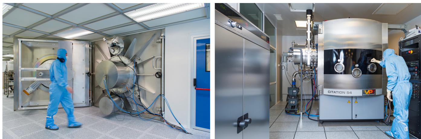
Figure 2: Large coating machines available at LMA-IP2I (Villeurbanne- France). Right: Large Ion Beam Sputtering chamber. Left: Large Ion Assisted Deposition chamber. © Cyril FRESILON / LMA / CNRS Photothèque.
